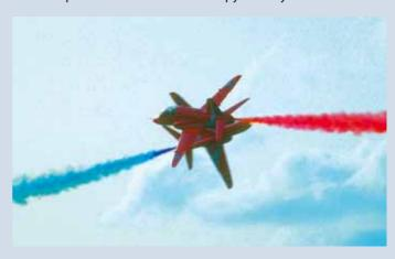
this elegant machine. The Hawk is powered by the two-shaft turbofan Rolls-Royce Turbomeca Adour engine developing a thrust of 2360 kg. The aircraft has two sealed tandem cockpits; this enables increased visibility for the instructor in the rear seat. Each cockpit is fitted with an ejection seat to abandon the aircraft on the ground. There are small horizontal planes on the sides of the fuselage ahead of the stabilizer to improve controllability of the aircraft at a high angle of attack.
